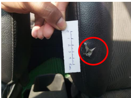
Fig. 2: Hole found at the corner of side seat of the driver.
